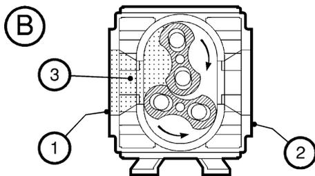
**Detail B** - As the impeller rotors rotate, gas (3) is drawn into the volume between the pump body wall and the rotors.
