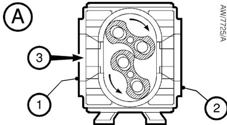
**Detail A** - Gas (3) enters the pump body through the inlet (1). In the pump body, the upper impeller rotor rotates clockwise, and the lower impeller rotor rotates anticlockwise (counterclockwise).
