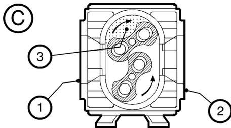
**Detail C** - As the rotors rotate further, gas (3) is trapped between the pump body wall and the rotors, and is transferred towards the outlet (2). The rotors rotate with precise timing to maintain the proper clearances, limiting gas back flow.
