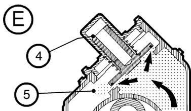
**Detail E:** bypass valve operation (only applicable to pumps with a bypass valve) - The optional integral bypass valve limits the pressure differential across the pump. During pump operation, if the compression creates an excessive pressure differential across the pump, the bypass valve (4) opens, to allow a portion of the compressed gases (5) to flow back towards the inlet side of the pump.
