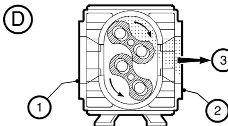
**Detail D** - As the rotors rotate further, the gas (3) is discharged through the pump outlet (2). The pump discharges four volumes for every full rotation of the drive shaft.
