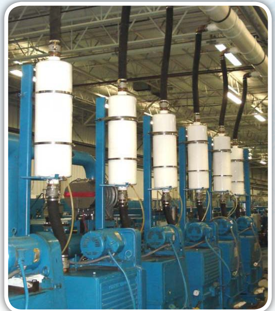
Edwards Vacuum Pump: Glass Coating Application Two-Stage Straight Through Discharge Oil Mist Eliminator
