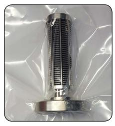
**CAUTION:** Do not remove the NEG from packaging until you are ready to install it into your vacuum system. The NEG's performance is degraded through long-term exposure to atmospheric conditions. Opening the NEG to a nitrogen environment is preferred but not required.
